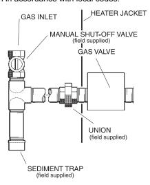
Figure 8. Gas Line Sediment Trap.
